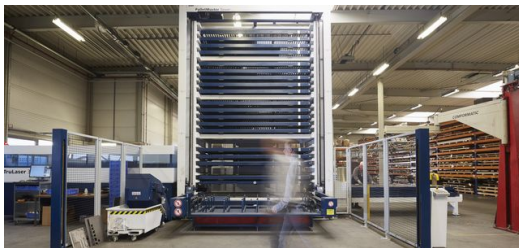
The PalletMaster Tower is flexible enough to meet any requirement. Stored in the 20 spaces at Koridon are all the types of sheet metal required for the lights-out shift (Photo: Claus Langer).
