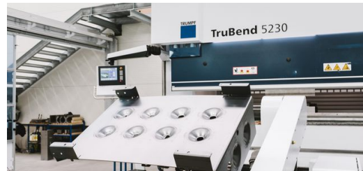
<p>For boiler plate production, half-shell-shaped recesses must be made in the plate. First a hard nut for the TruBend Cell 5000. Today, the bending cell handles the forming process fully automatically, saving a lot of time.</p> – Stefan Fuertbauer
