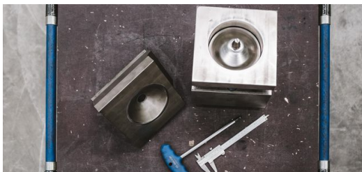
<p>The special tools developed by TRUMPF in Pasching especially for PNH, enables to automate the rigging of semicircular, bowl-shaped depressions required for the boiler plate manufacturing process.</p> – Stefan Fuertbauer
