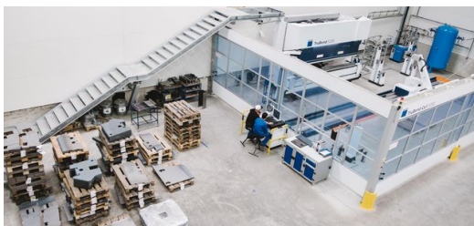
<p>With its 230-tonne press force, the TruBend Cell 5000 can process components of 3000 x 1500 millimeters conveniently.</p> – Stefan Fuertbauer
