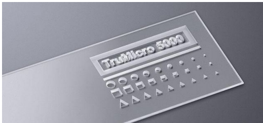
With regard to watch crystals and watch faces made of sapphire: the cold processing generates no heat, thus preventing microscopic cracks that might weaken such components as this thin sapphire platelet. Picture: TRUMPF
