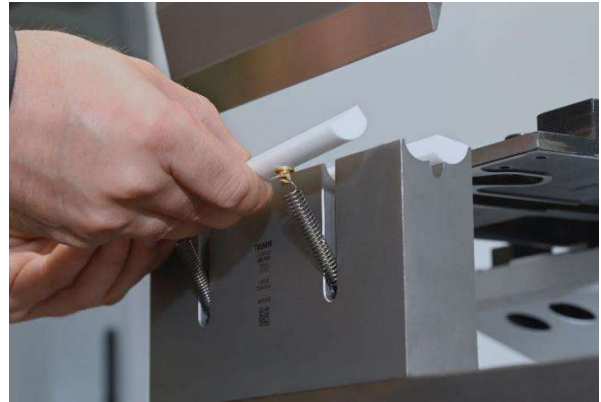
No tools needed for changing the plastic jaws
