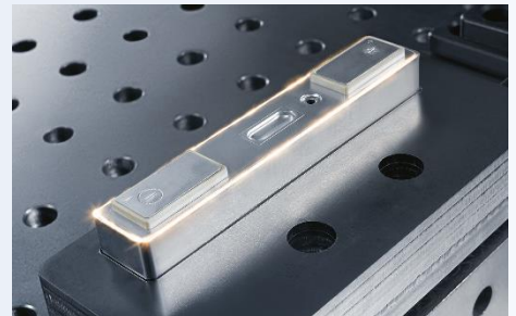
Welding a battery can cap Material: aluminum
