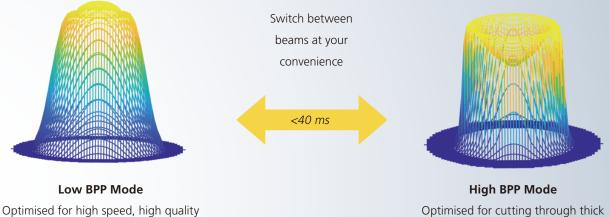
Optimised for cutting through thick metal sheets at high speed, producing an excellent surface finish
