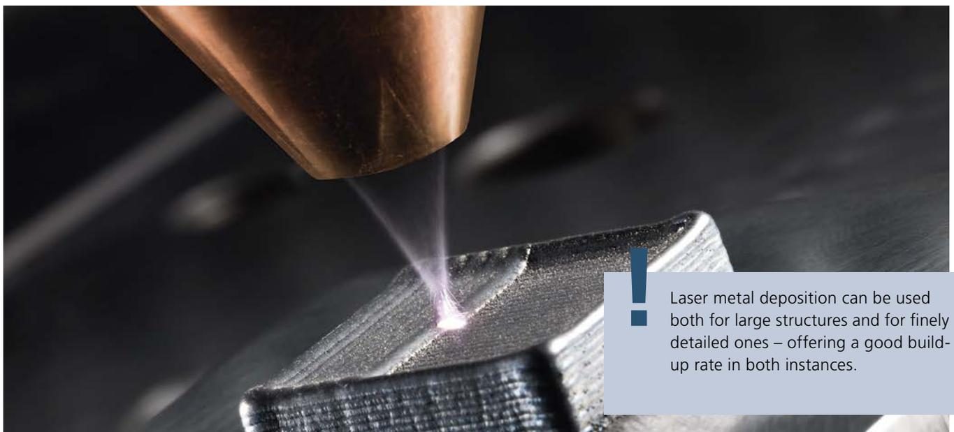
Laser metal deposition can be used both for large structures and for finely detailed ones – offering a good build-up rate in both instances.
