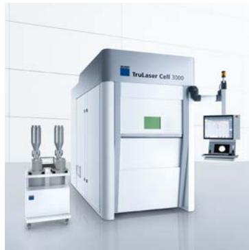
From prototype to full-scale production: with this 3-in-1 machine, you can process small and medium-sized components extremely efficiently. The machine is equipped for laser metal deposition (LMD) as well as laser cutting and welding in 2D and 3D. Process adapters make it particularly easy to switch between techniques.
