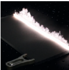
Test application: high-speed ablation of a polymer matrix in compound bipolar plates for fuel cells.
