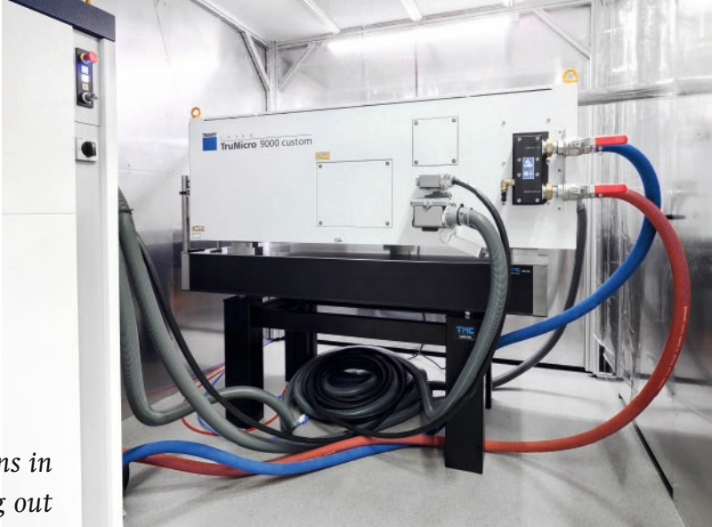
Test application: high-speed ablation of a polymer matrix in compound bipolar plates for fuel cells.
