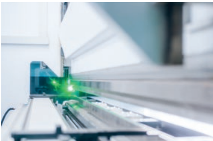
Speed: The machine bends a six-meter workpiece in just 37 seconds – including loading and unloading.
