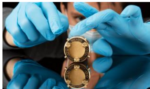
Sample carrier for the rapid characterization of material samples and quantum electronic components at sub-Kelvin temperatures (-272 °C) with magnetic refrigerators from kiutra.
