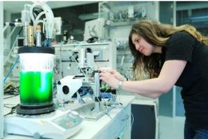
**Algae are conveyed to the sensor automatically and continuously through special microfluidic components made by Festo.**
