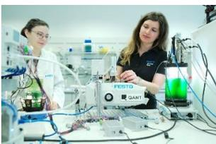
**One of the biggest challenges is how to accurately determine the amount of biomass. To do this, Festo relies on quantum sensor technology from Q.ANT.**
