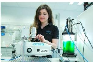
**A Festo engineer connects up the microfluidic pumps that deliver the algae fluid to the Q.ANT sensor.**
