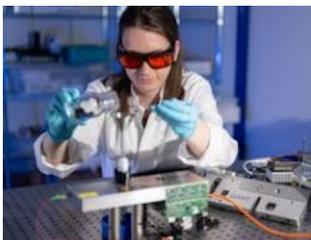
**A Q.ANT specialist performs test measurements on coffee grounds. Liquids, gases and powders can all be measured by quantum sensors.**
