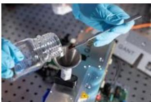
**The quantum sensor can simultaneously measure the size, shape and speed of individual particles in a powder passing through the sensor.**
