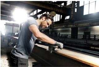
The new TruTool TKA 1500 edge trimmer from TRUMPF produces polished metal chamfers up to 15 millimeters long.
