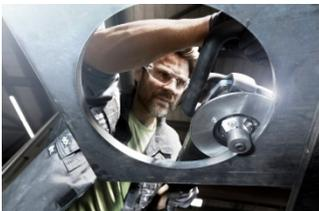
Operators can use the dTKA 1500 to apply radii of between two and four millimeters.
