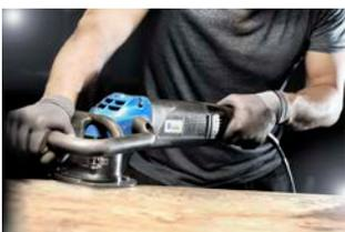
Thanks to the ergonomically designed guide and motor handles, operators can use the new edge trimmer for long periods without getting tired, maintaining high-quality chamfers from start to finish.
