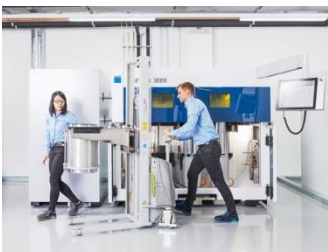
TRUMPF additive manufacturing Employees remove the cylinder with the component from the 3D printer for further processing.
