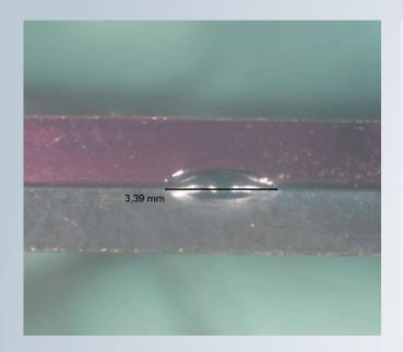
Round parts are often contour-welded with fixed optics and the mating parts are rotating at up to 25 m/min under the laser beam. Housings are welded quasi-simultaneously at speeds up to 15 m/s with scanner optics. The high speeds require a scanner with good contour precision. Joint pressure Weld seam Weld seam Cap < 150 µm
