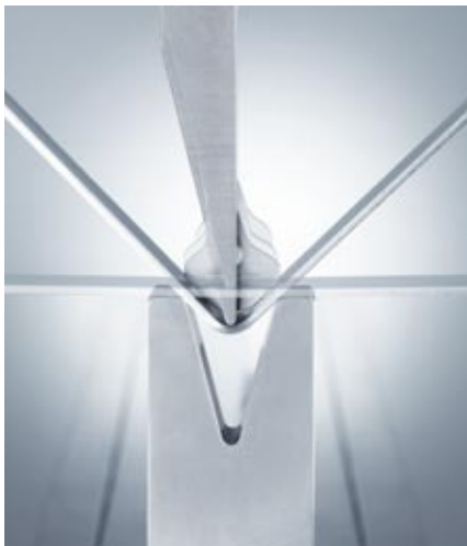
Automatic bending with angle sensor ACB.
