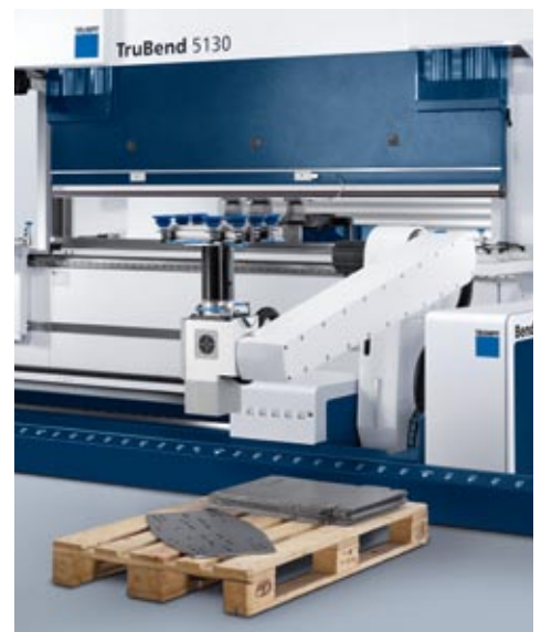
BendMaster (60) collecting fine positioning data.
