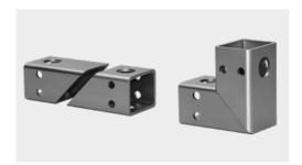
Thanks to bevel cuts of up to 45°, you can further process corner connections more quickly – with optimal material utilization.
