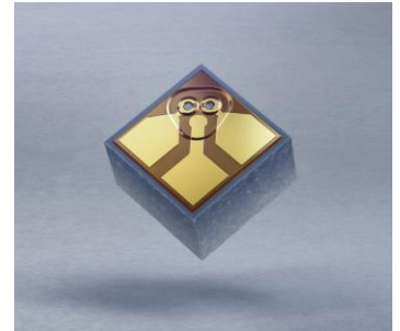
Chip die – two 850 nm VCSELs with single integrated photodiode for high-volume self-mixing interferometry sensing applications and integrated speed sensors
