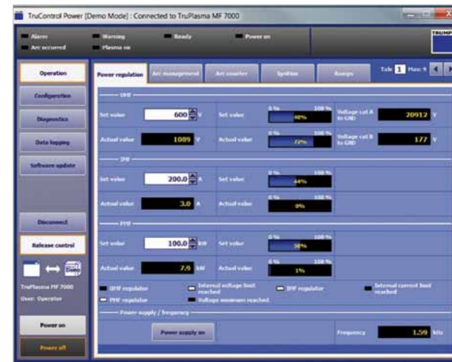
The convenient TruControl Power operating software features comprehensive configuration and diagnosis functions.
