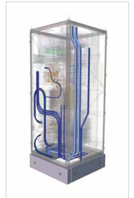
One hundred percent water cooling is not only highly effective but a very clean cooling method as well. The risks of air cooling (for example contamination or corrosion due to salty air) are avoided.
