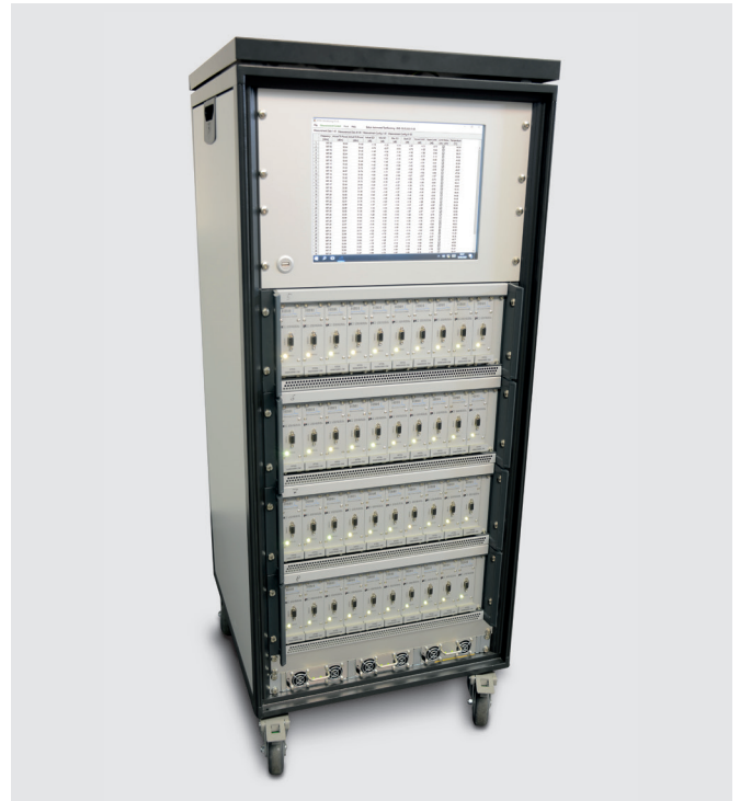
Figure 2: Complete 80-Channel HTOL Rack
