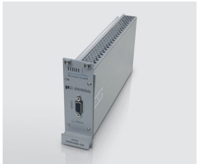
Figure 1: Single 2-Channel HTOL Module
