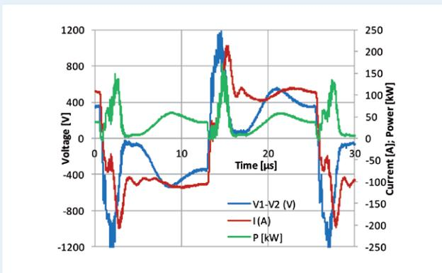
Fig. 4: Example of current, voltage and instantaneous power with a square wave generator; target and process conditions as in Figure 3 (40kW, 490V, 100A).
