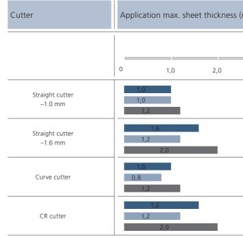
Steel (400 N/mm<sup>2</sup>) Stainless steel (600 N/mm<sup>2</sup>) Aluminium (250 N/mm<sup>2</sup>)
