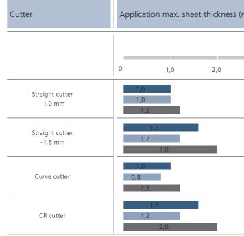
■ Steel (400 N/mm<sup>2</sup>) ■ Stainless steel (600 N/mm<sup>2</sup>) ■ Alu (250 N/mm<sup>2</sup>) ■ Spiral ducts
