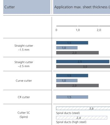
■ Steel (400 N/mm<sup>2</sup>) ■ High steel (600 N/mm<sup>2</sup>) ■ Aluminium (250 N/mm<sup>2</sup>) ■ Spiral ducts
