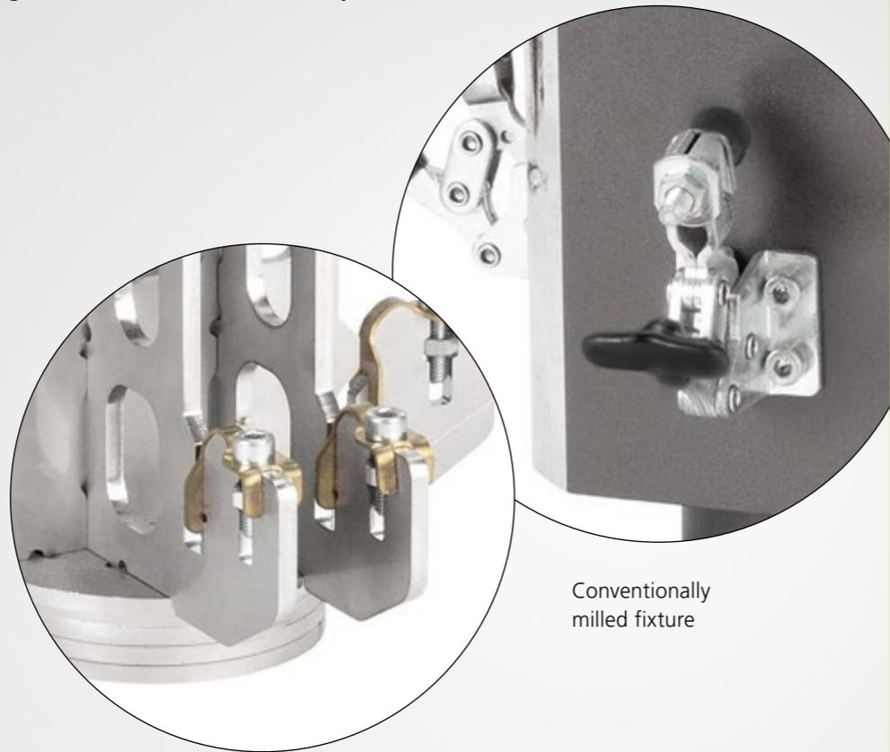
Optimized fixture made out of sheet metal
