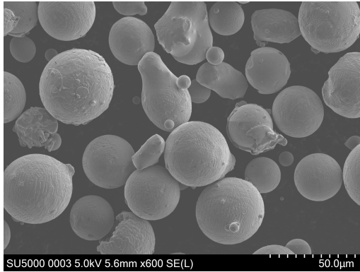
Figure 8: In625 powder by Oerlikon Metco. PSD: 15-45 μm. SEM magnification: 600x.
