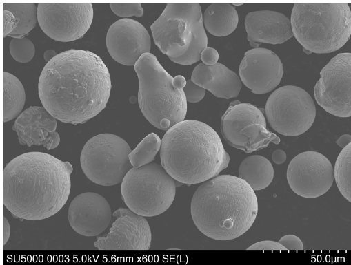
Figure 2: In625 powder by Oerlikon Metco. PSD: 15-45 μm. SEM magnification: 600x.
