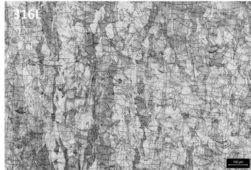
Figure 6: Microstructure of 316L: no heat treatment
