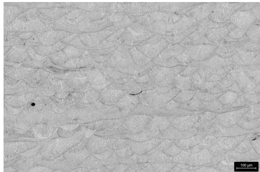
Figure 12: Microstructure of H13: no heat treatment
