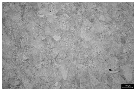
Figure 8: Microstructure of Dievar: no heat treatment
