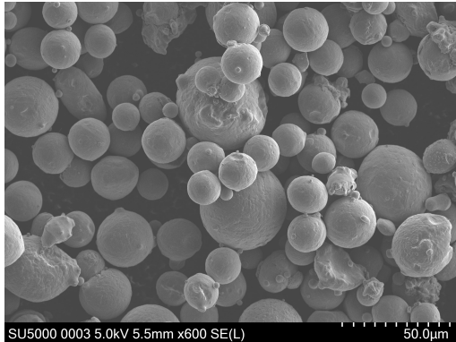
Figure 10: H11 powder by Höganäs. PSD: 10-45 μm. SEM magnification: 600x.
