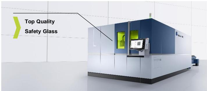
TRUMPF laser cutting machines are also equipped with professional safety glass of "Optical Density" (OD) 6, which offers top protection, and the residual laser is only 0.0001%.
