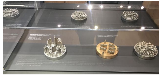
Substrate plates with 3D-printed dental prosthesis.
