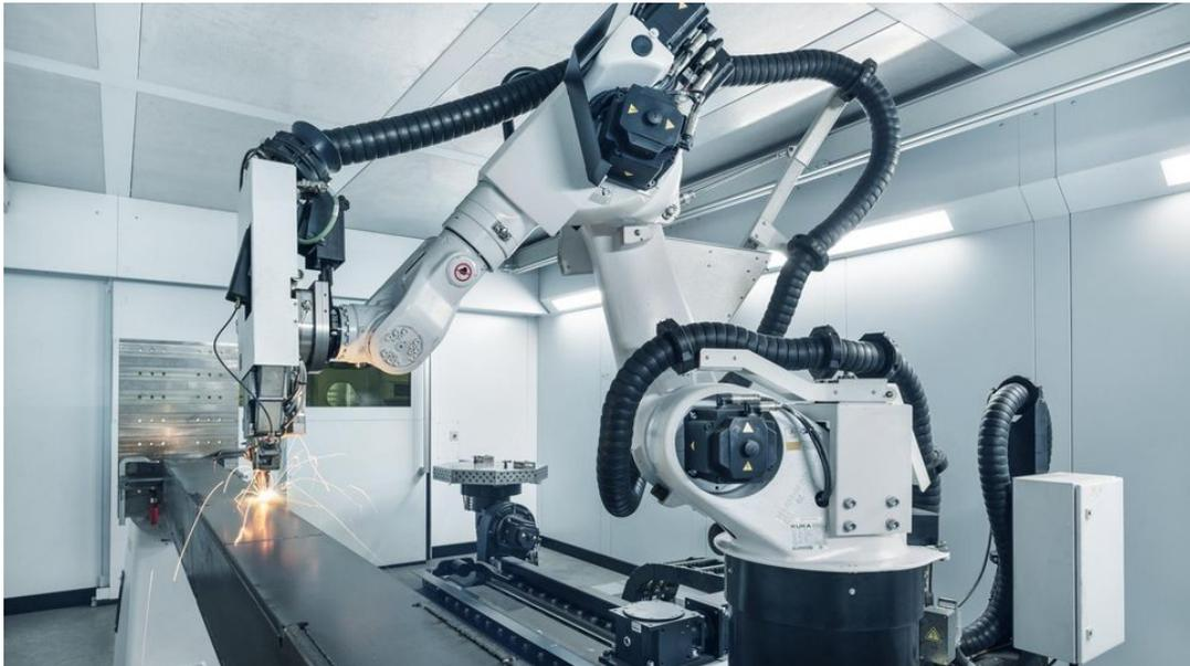
The TruLaser Weld 5000 large format machine at Böhmer Systemtechnik is equipped with a KUKA robot on a linear axis and a turnover positioner, allowing it to cover a working area 4 meters long and 1.5 meters wide. The rotate-and-tilt positioner gives users the flexibility to weld the occasional small part between a series of larger ones.
