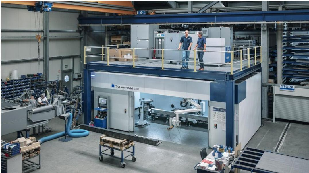
To save space, all the TruLaser Weld 5000's peripherals and system technology are positioned on a dedicated enclosure above the machine.
