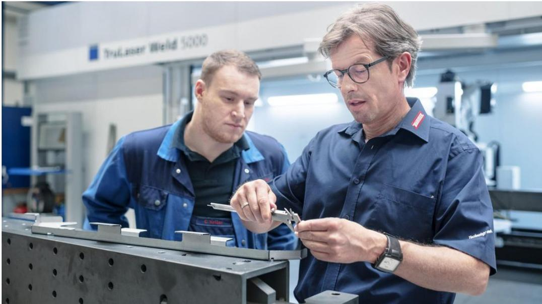
Deep penetration welding with a laser involves far less heat input than conventional welding methods – and that means less distortion. Josef Böhmer (right): “Parts nowadays have to be made to such fine tolerances, especially in formwork construction. So we save a lot of time by not having to straighten them after welding!”
