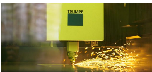
In March, FBT workers started using their new TruLaser 3030 to cut thin sheets and blanks to size. Image: Stephen Duscher
