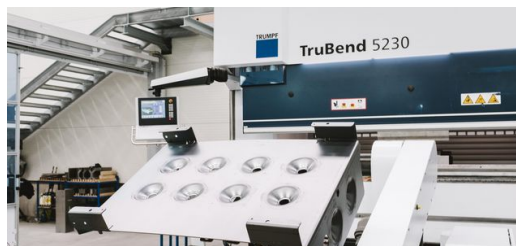
For boiler plate production, half-shell-shaped recesses must be made in the plate. First a hard nut for the TruBend Cell 5000. Today, the bending cell handles the forming process fully automatically, saving a lot of time.
