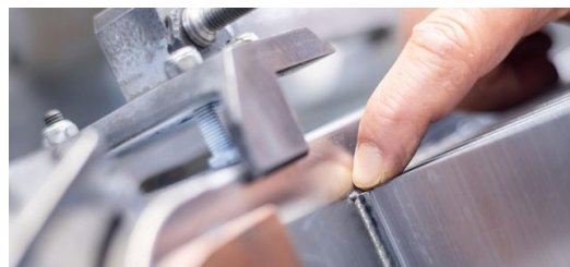
The welded seams of the housing must be completely sealed so that the electronics of the inverter are optimally protected against environmental influences.
