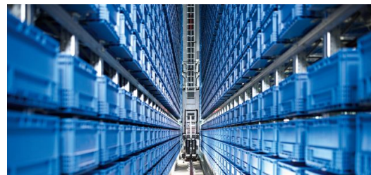
The automated small parts store (AKL) keeps products in 23,000 shelf spots. Picture: Claus Morgenstern
