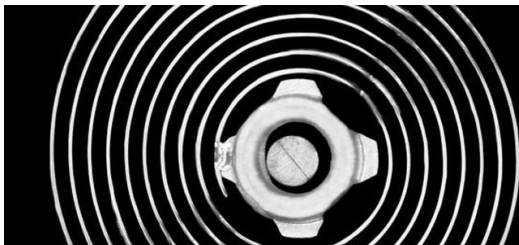
One of the first industrial laser applications: laser-welded watch springs. Picture: TRUMPF
