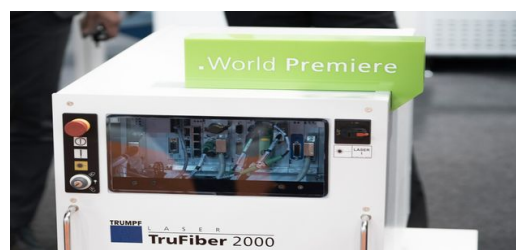
The fiber-based solid-state laser TruFiber 2000 celebrated its world premiere at the LASYS 2018. Because this laser has a compact laser design, flexible interfaces to all common fieldbus systems, and the maximum laser safety rating with Performance Level 'e', it also contributes to easy integration. Image: Lorenz Buchwald
