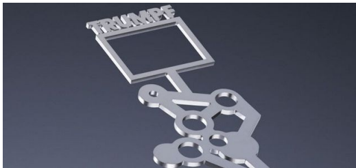
In fusion cutting, the material melts into the kerf while shielded by an inert gas and the molten material is forced out by the gas pressure. Picture: TRUMPF
