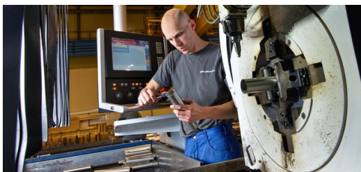
Each day one or two of the programmers are fully occupied with preparations for two-shift operations. The TruTops Tube Software makes possible exact calculation of cutting geometries. Picture: Escherich Fotografie
