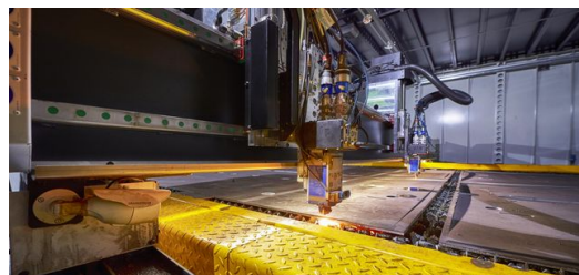
Two cutting heads equipped with 0.5 and 1 mm fibers can cut individually or in parallel (Photos: Norbert Voskens).
