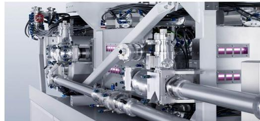
The TRUMPF Laser Amplifier is based on the technology used for the continuous wave CO<sub>2</sub> laser and operates in a performance range exceeding ten kilowatts. In five amplifier stages it boosts a CO<sub>2</sub> laser pulse of just a few watts of mean power more than 10,000 times, outputting more than 30 kilowatts of mean pulse power.
