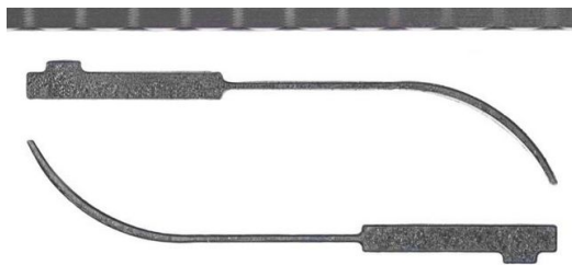
Picosecond lasers cut the most minuscule precision mechanical components; here, a second-stop spring for wristwatches made of 0.05 millimeter thick stainless steel. Picture: TRUMPF
