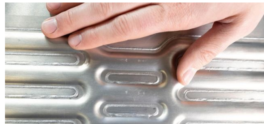
<p>In the folding-box concept developed by BENTELER for a stainless steel battery housing, the patented TRUMPF solution BrightLine Weld ensures spatter-free processing and high-strength gas- and helium-tight weld seams, even in rapid series production.</p>
