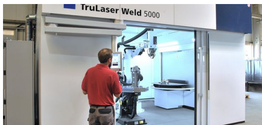
Significant savings: sheet metal fabricator Schink operates its TruLaser Weld 5000 laser welding cell and TruLaser 3040 laser cutting machine in what's known as a laser network. That means the two systems share a 4-kilowatt TruDisk 4001 solid-state laser source. Image: Peter Klingauf
