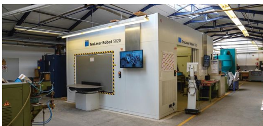
Hey Mr. Robot: The TruLaser Robot 5020 helps Gefinal perform challenging welding jobs.
