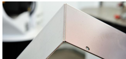
"Tolerant" laser welding is essential for components that have gaps or awkward overlaps. The TruLaser Weld 5000 offers this capability with its optional FusionLine feature. Image: Peter Klingauf
