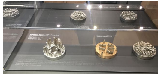
Substrate plates with 3D-printed dental prosthesis.
