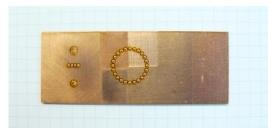
Regardless of whether the surface is oxidized, ground, sandblasted, rough, or polished to a high gloss, a green laser beam makes it possible to create welding seams in copper which are always of uniform quality. Picture: TRI IMPE
