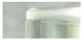
Lateral view: Laser-welded protective caps are more than twice as strong as conventionally joined caps in breakage tests.
