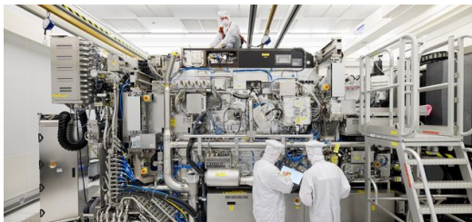
<p><span lang="EN-US">ASML employees working on a new generation of the EUV lithography system NXE3400B.</span></p> – ASML
