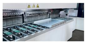
The concept for machining perforated sheets is well thought out. Suction cups, or optional magnetic clamps, can be positioned as desired and secure the sheets firmly. (Picture: KD Busch)
