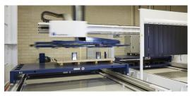
The SheetMaster is entrusted with loading and unloading the machine. It sorts the parts and lays them on the cart or pallet. (Picture: Claus Langer)
